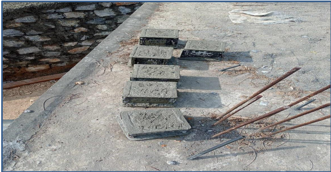
Preparation of Cube for Lab Test
