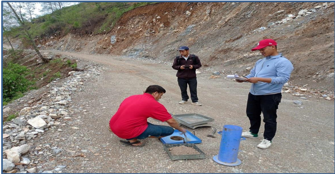
field density check by sand replacement method
